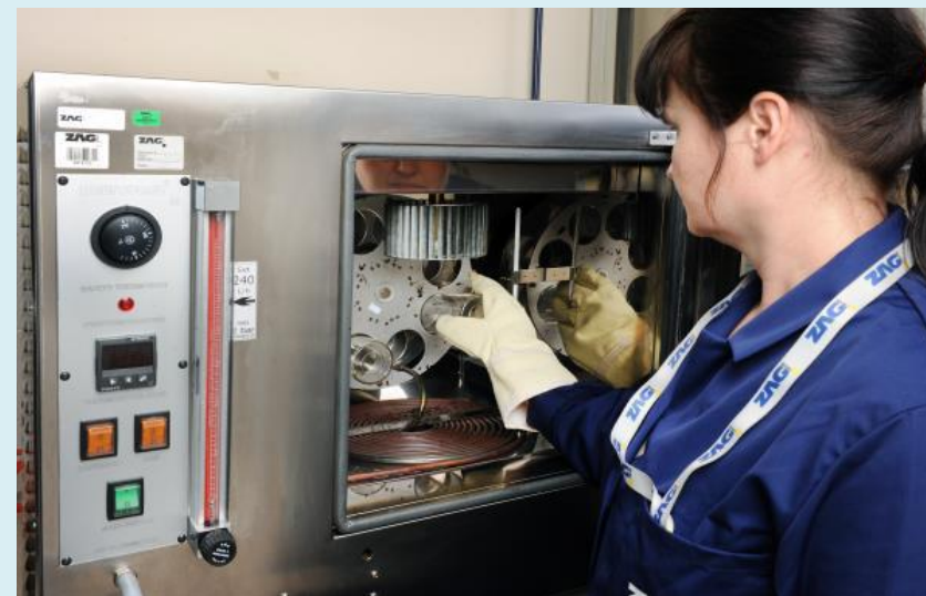
SIST EN 12607-1: Določanje odpornosti proti utrjevanju pod vplivom toplote in zraka RTFOT Determination of the resistance to hardening under influence of heat and air (RTFOT)
