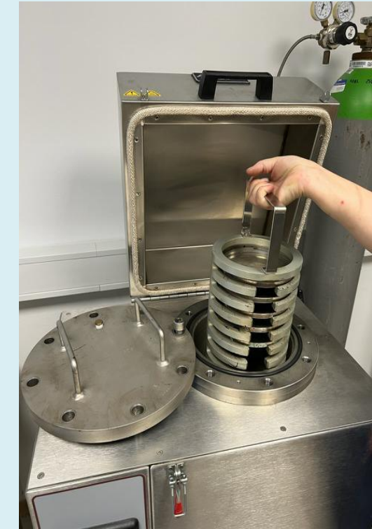
SIST EN 14769: Bitumen in bitumenska veziva – Pospešeno staranje v tlačni posodi Accelerated long-term ageing conditioning by a Pressure Ageing Vessel (PAV)
