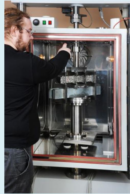
SIST EN 12607-1: Določanje odpornosti proti utrjevanju pod vplivom toplote in zraka RTFOT Determination of the resistance to hardening under influence of heat and air (RTFOT)
